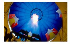
A hot air balloon must be filled with air and the air must be heated for the balloon to be able to lift off the ground. The air has to be kept warm of the balloon will fall.
